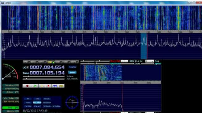
Example of saturation and intermodulation with HF converter at FCD input
