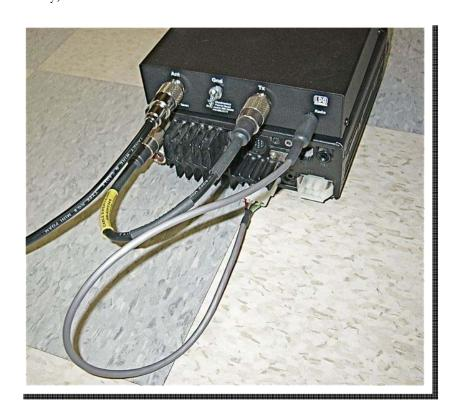
"Tuner" jack on the rear of the Icom transceiver.
